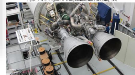
Figure 4. Antares First-Stage Core with Two AJ26 Engines Installed
